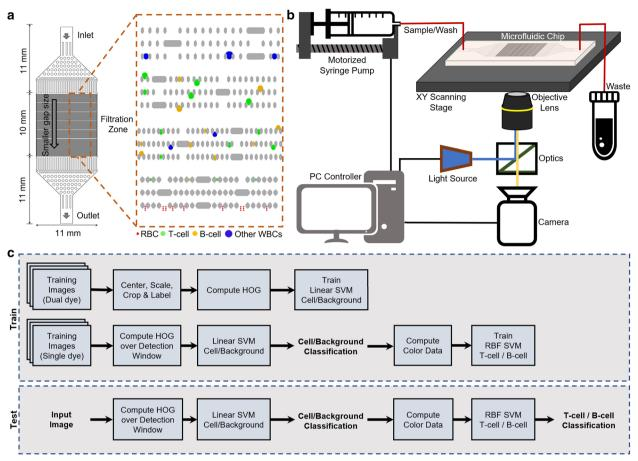
Fig. 1 Overview of the proposed system. a Design of the microfluidic chip, blood is pumped into the device via inlet port. Due to the difference in size and deformability, leukocytes will be trapped in different zones. b Experiment setup. c Block diagram of cell detection framework using machine learning method
