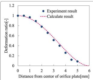
Fig. 13 Comparison of calculated result and actual deformation ratio value
