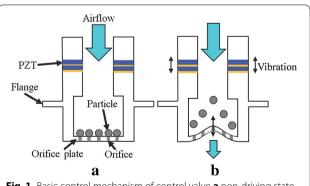
**Fig. 1** Basic control mechanism of control valve **a** non-driving state, **b** driving state
