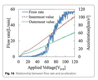
was because the particles opened and closed irregularly. When the flow rate increases, the number of moving particles increases, and the flow rate varies temporally. Optimizing the orifice size, the number of orifices and the particle size could solve this problem.
