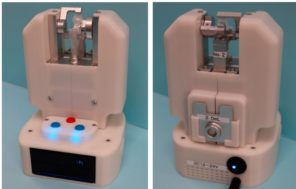
Fig. 9 Overview of a prototype of the proposed manually operated microtube automatic capper/decapper system
