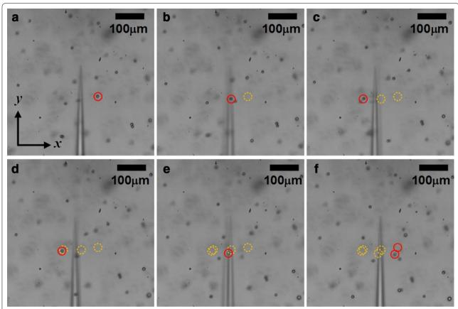
**Fig. 6** Rotational flow by the circular motion at 100 Hz. The microbead is tracked when the end-effector is rotating in 100 Hz. **a** Initial position, **b** 0.028 s, **c** 0.056 s, **d** 0.084 s, **e** 0.112 s, **f** 0.14 s
