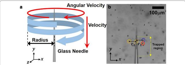
Fig. 7 Measurement method of rotational stream in 3D space. **a** Measurement method of flow velocities. **b** Trajectory of a microbead by the rotational stream
