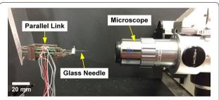
**Fig. 3** Experimental setup for observing the motion of the end effector
