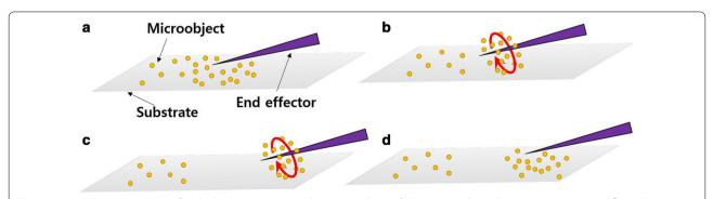
Fig. 10 Manipulation procedure of multiple objects. **a** Approach to target objects. **b** Trap target objects by generating rotational flow. **c** Transport targets by moving stage. **d** Place targets to the desired position by stopping the end effector's motion
