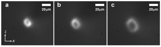
Fig. 4 High-speed circular motion of the end effector for different amplitudes. The frequency is 100 Hz and the amplitude is **a** 12 μm, **b** 15 μm, **c** 21 μm
