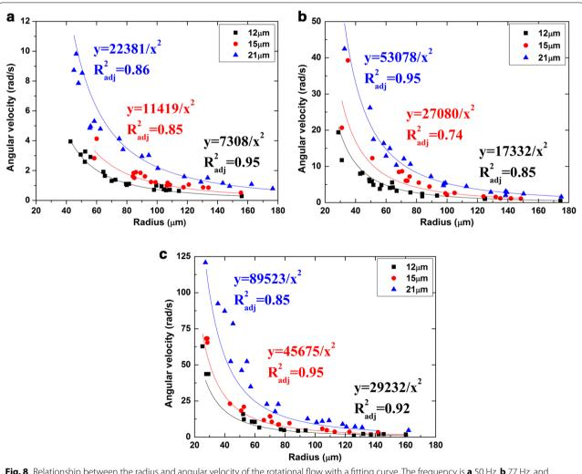
Fig. 8 Relationship between the radius and angular velocity of the rotational flow with a fitting curve. The frequency is **a** 50 Hz, **b** 77 Hz, and **c** 100 Hz
