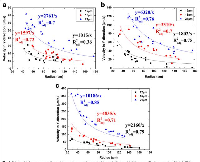
Fig. 9 Relationship between the radius and the velocity toward the root of the end-effector with fitting curve. The frequency is **a** 50 Hz, **b** 77 Hz, and **c** 100 Hz
