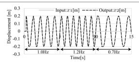
(a) Examples of the input and the output of the controller (The frequencies are 1.0 Hz, 1.2 Hz, and 0.7 Hz during 0-5 s, 5-10 s, and 10-15 s respectively)
