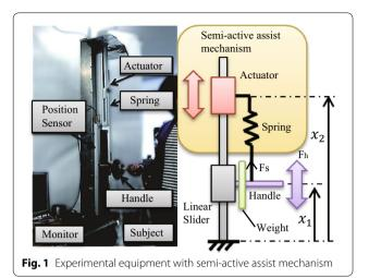
and the assist force  $F_s$  generated by the semi-active assist mechanism can be expressed as follows:
