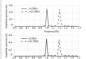
(b) Examples of the frequency entrainment characteristics of the controller
